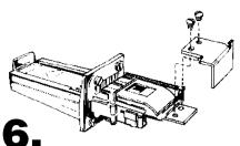
Open control panel and rest it on the bottom edge of the opening. Attach slide extension (with flange pointing down) to one of the coin-slide mechanisms. Insert the coin-slide mechanism through the opening to the left of the control panel.
